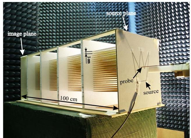
FIG. 1. (Color online) Photograph of the wire medium lens:  $21 \times 21$  array of parallel 1-m long aluminum wires. The period of the array is 1 cm. The radius of the wires is 1 mm. The source in the form of a crown is adjacent to the front interface of the lens. The source is fed by a coaxial cable connected to a network analyzer. A small electric probe used for near field scan is shown together with the supporting arm.
