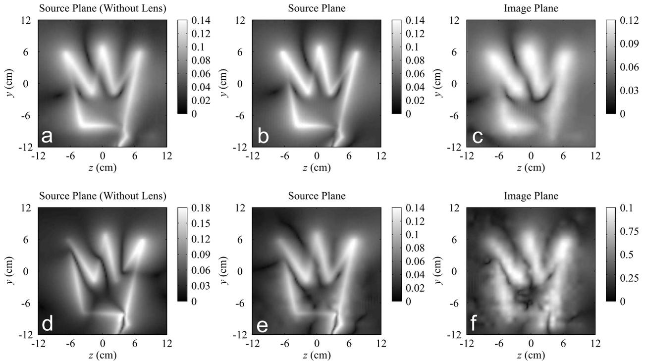
FIG. 2. Results of the near-field scan at the source plane (2 mm away from the front interface of the lens) without (a) and with (b) the wire medium lens and (c) at the image plane (2 mm away from the back interface of the lens) at 894 MHz. (d), (e), and (f) are the same as (a), (b), and (c) but at 1038 MHz.
