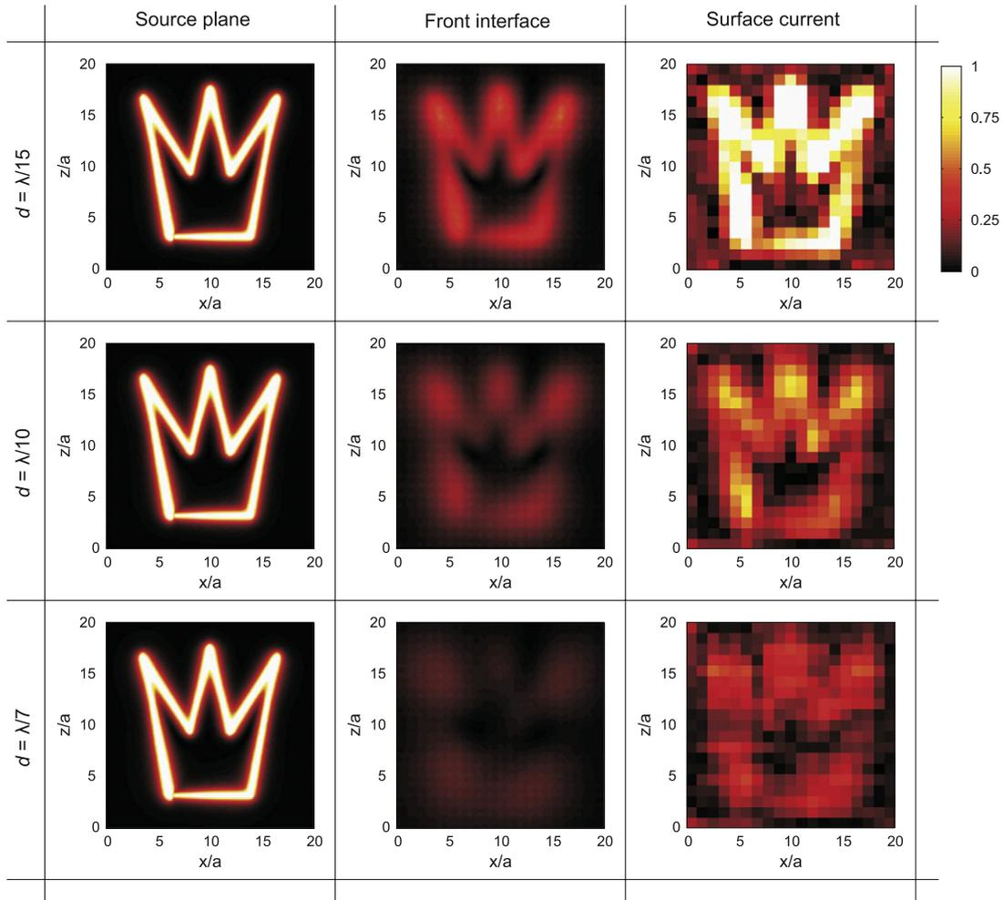
**Figure 3.** Normalized distributions of the y-component of the electric field at the source plane and the front interface, and the current density at the internal image plane of the wire medium for different distances between the source and the wire medium calculated from CST simulations of the physical structure.
