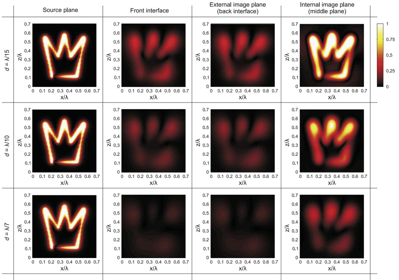
**Figure 2.** Normalized distributions of the  $y$ -component of the electric field at the source plane, the front interface, and the electric displacement at the internal image plane of the wire medium for different distances between the source and the wire medium calculated from spatially dispersive FDTD simulations.
