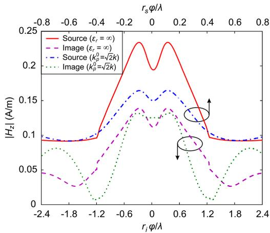
**Figure 10.** Comparison of magnetic field distributions in the source and image planes of two hyperlens structures with  $\epsilon_r = \infty$  and  $k_p^0 = \sqrt{2}k$ . In both cases,  $L = \lambda$ .
