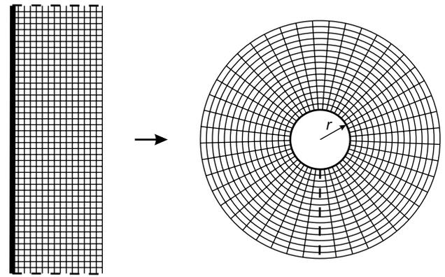
**Figure 3.** Mapping of a 2D array to the FDTD grid in cylindrical coordinates. The thick solid/dashed lines indicate the same array of elements.
