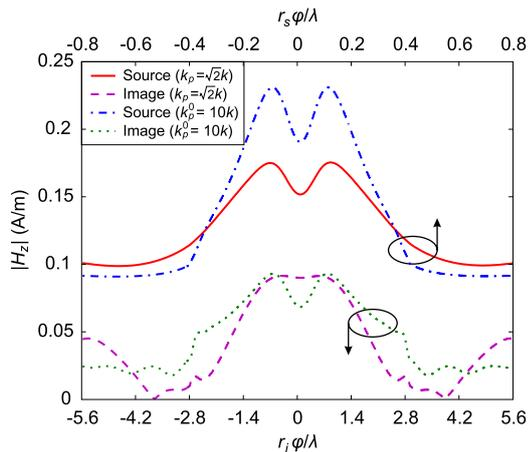
**Figure 12.** Comparison of magnetic field distributions in the source and image planes of two hyperlens structures with  $k_p^0 = \sqrt{2}k$  and  $10k$ . In both cases,  $L = 3\lambda$ .
