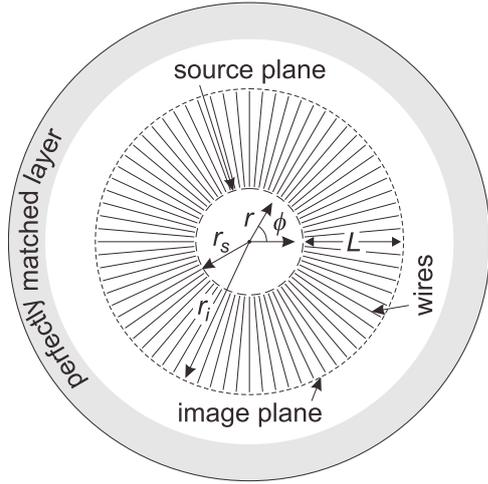
**Figure 5.** The 2D FDTD simulation domain in cylindrical coordinates for the modeling of a hyperlens formed by a tapered array of wires.
