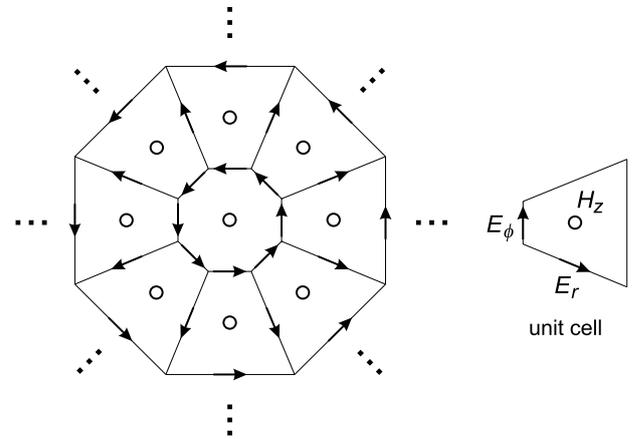
**Figure 4.** Layout of the FDTD grid in cylindrical coordinates in the vicinity of the origin, where the  $H_z$  component is located and treated separately.
