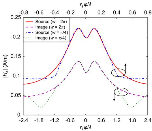
**Figure 8.** Comparison of magnetic field distributions at the source and image planes of two hyperlens structures with angular widths of  $w = 2\pi$  and  $\pi/4$ . In both cases,  $k_p^0 = 10k$ .
