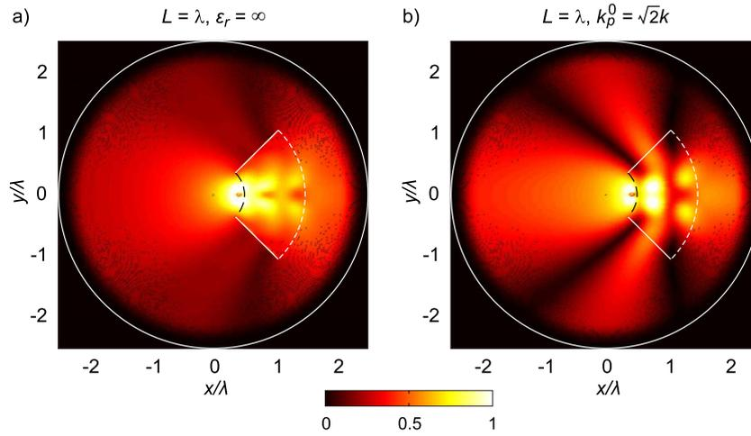
**Figure 9.** Normalized magnetic field distributions for two hyperlens structures with (a)  $\epsilon_r = \infty$  and (b)  $k_p^0 = \sqrt{2}k$ . In both cases,  $L = \lambda$ .
