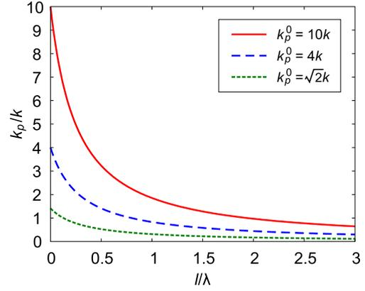
**Figure 6.** Normalized value of  $k_p$  versus the location within the hyperlens (with reference to the inner interface), where  $k_p^0$  is the value of  $k_p$  at the inner interface.
