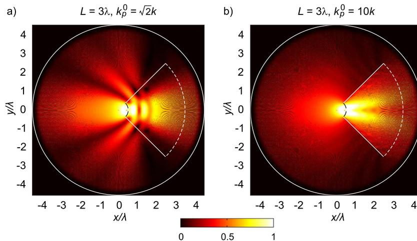
**Figure 11.** Normalized magnetic field distributions for two hyperlens structures with (a)  $k_p^0 = \sqrt{2}k$  and (b)  $k_p^0 = 10k$ . In both cases,  $L = 3\lambda$ .
