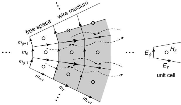
**Figure 2.** A partial grid layout in cylindrical FDTD domain for the modeling of a hyperlens formed by a tapered array of wires. The dashed arrows indicate the dependency between adjacent field components.
