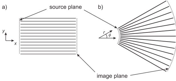
**Figure 1.** (a) The 2D view of a parallel wire medium as a transmission device. (b) The 2D view of a hyperlens formed by a tapered array of wires which can be conveniently represented in cylindrical coordinates.
