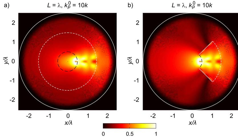
**Figure 7.** Normalized magnetic field distributions calculated from cylindrical FDTD simulations for two hyperlens structures with angular widths of (a)  $w = 2\pi$  and (b)  $w = \pi/4$ .
