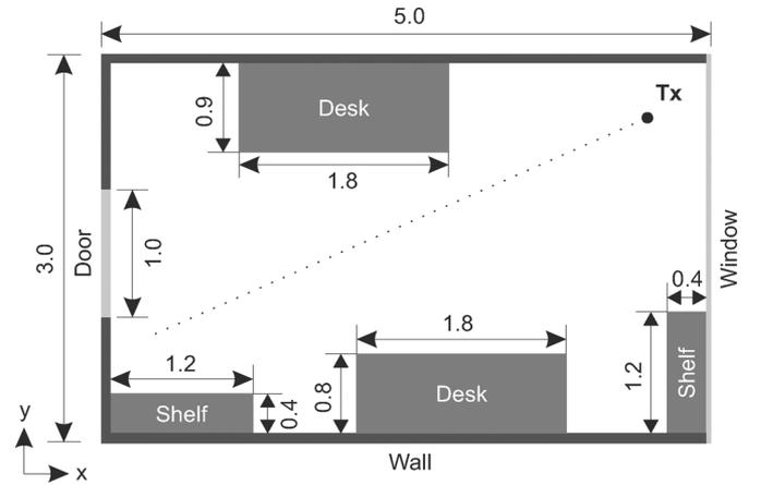
Fig. 3. Layout of the subband FDTD simulation domain (unit: m).
