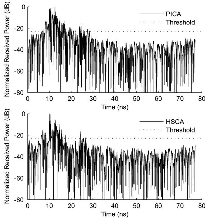
Fig. 5. PDPs calculated from combined time domain CIRs at 3 m to Tx for different base station antenna cases. A threshold of  $-23$  dB for detecting the MCs is also shown.
