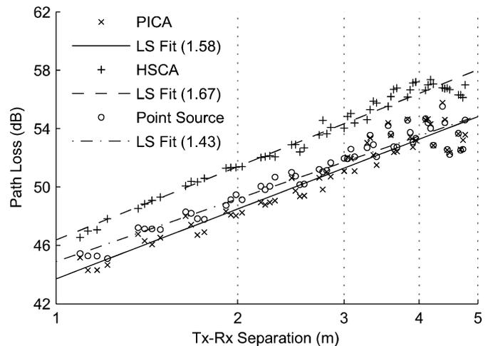
Fig. 6. Path loss at 1 to 5 m to the transmitter for different base station antenna cases. The least square (LS) fitted lines and the values of path loss exponent (in brackets) are also shown.
