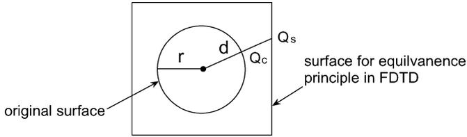
Fig. 1. Demonstration of the original circular surface where the antenna radiation patterns are calculated and the square surface for applying the equivalence principle in FDTD mesh.  $Q_c$  and  $Q_s$  are the example field points where the transformation is performed.
