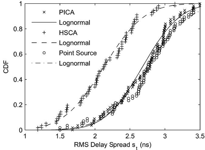
Fig. 7. CDF of rms delay spread for using PICA, HSCA, and PS as base station antennas, respectively.
