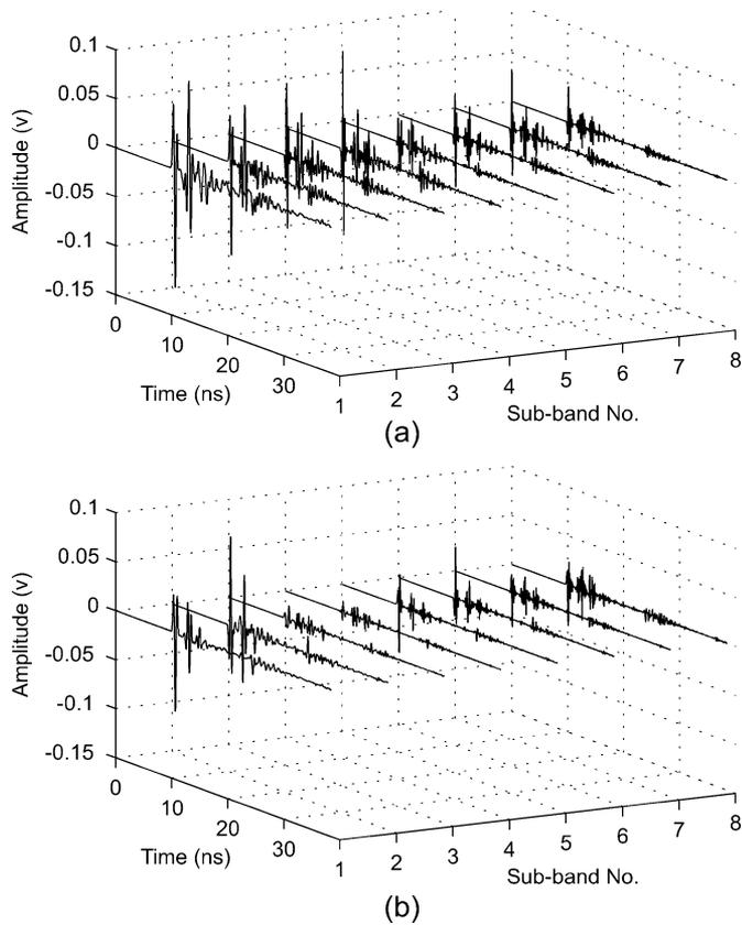
Fig. 4. Time domain CIRs at 3 m to Tx at different subbands using (a) PICA and (b) HSCA as base station antennas.
