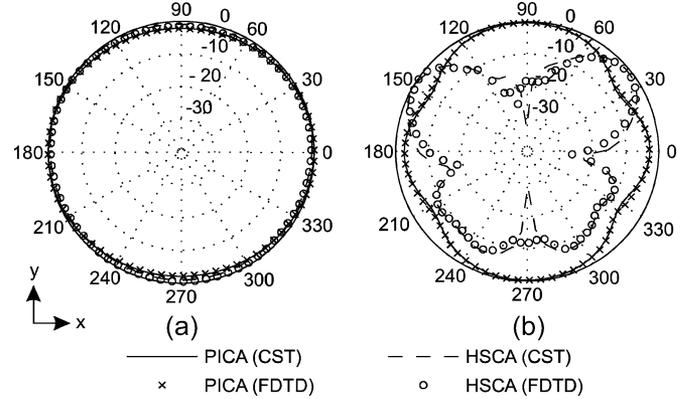
Fig. 2. Comparison of normalized E-field radiation patterns of PICA and HSCA at (a) 3.5 and (b) 10.5 GHz calculated from CST microwave studio modeling the actual antenna and from FDTD applying the equivalence principle.
