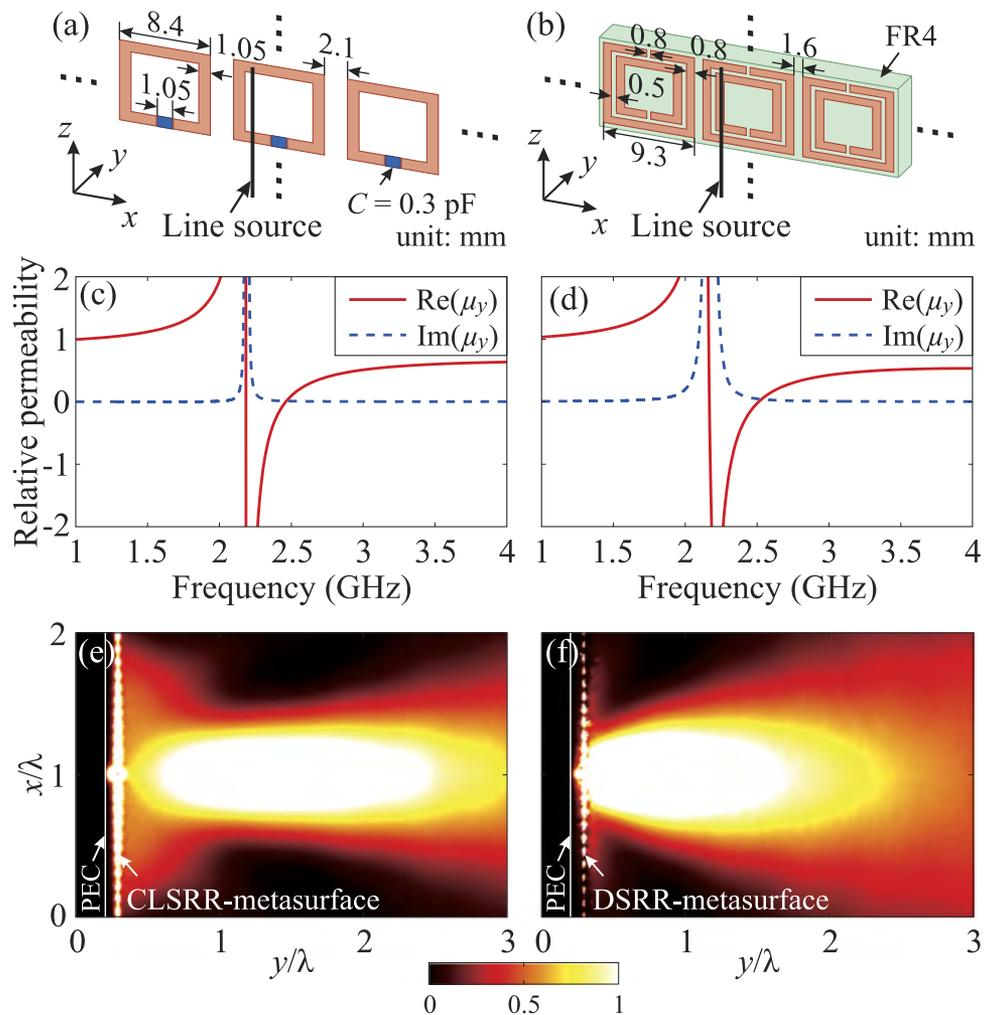
FIG. 2. Microwave metasurfaces formed by a single layer of (a) capacitively loaded SRRs (CLSRRs), and (b) substrate-backed double SRRs (DSRRs). Retrieved effective permeability for (c) the CLSRR-HMS, and (d) the DSRR-HMS. Distributions of electric field intensity for (e) the CLSRR-HMS and (f) the DSRR-HMS, both at 2.45 GHz.
