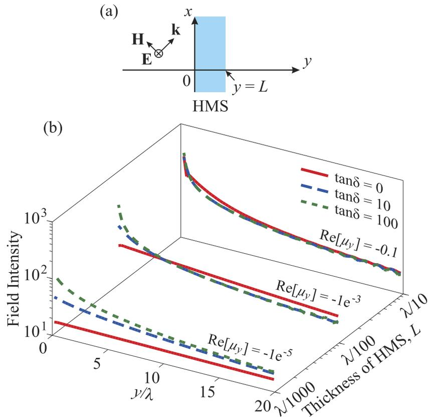
FIG. 1. (a) The two-dimensional domain for the transmission analysis of HMS. (b) The variations of electric field intensity along the  $y$ -direction for different thicknesses and amount of losses of HMS. In all cases,  $\mu_x = 1$ .
