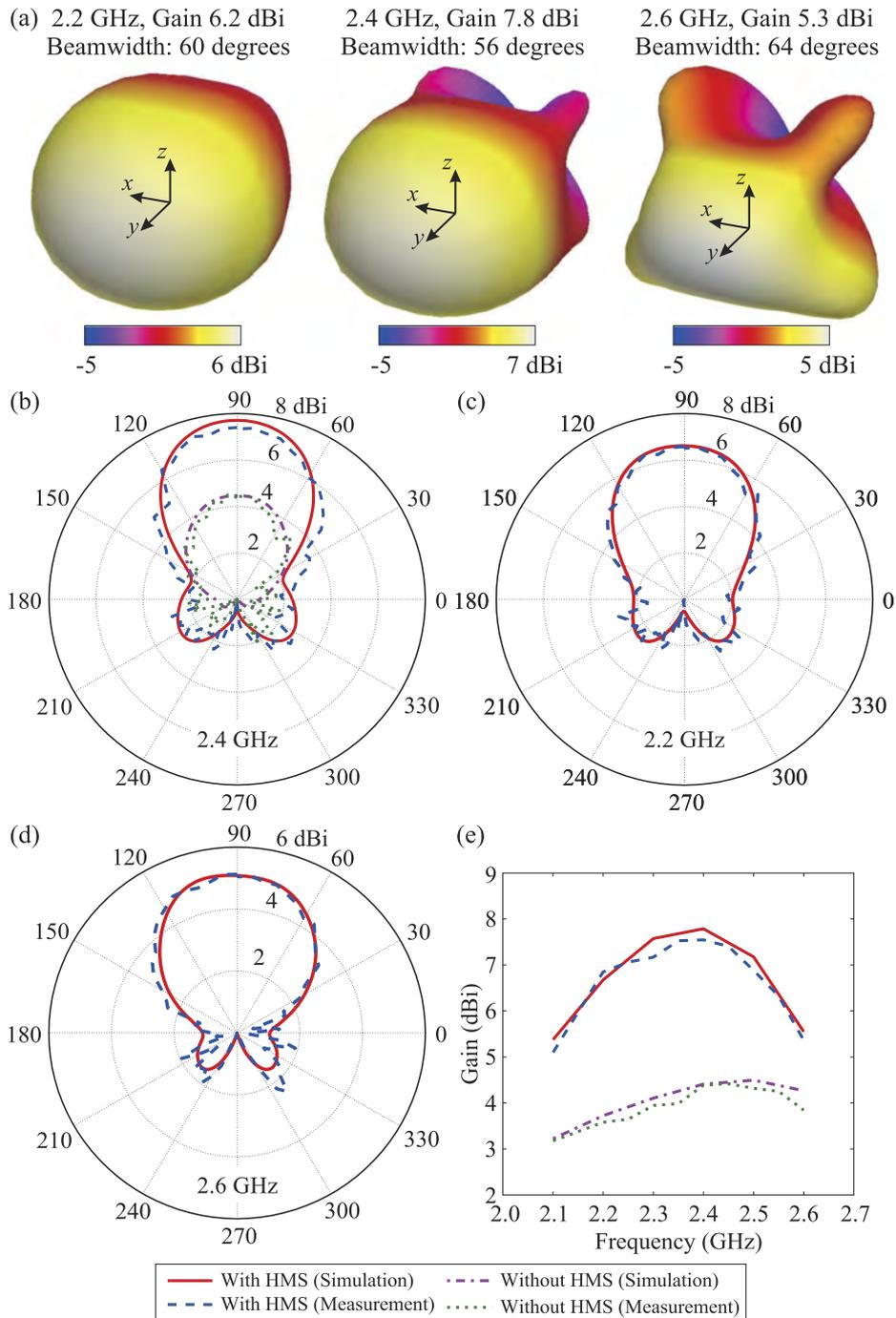
FIG. 4. (a) The radiation patterns of the proposed antenna at 2.2, 2.4 and 2.6 GHz from FEM simulations. (b) Comparison between simulated radiation patterns and measurement results at 2.4 GHz in the  $x$ - $y$  plane for the cases of with and without the use of the DSRR-HMS. Comparison between simulated and measured radiation patterns at (c) 2.2 GHz and (d) 2.6 GHz with the use of the DSRR-HMS. (e) Comparison between simulated and measured antenna gain in the frequency range of 2.1 - 2.6 GHz.
