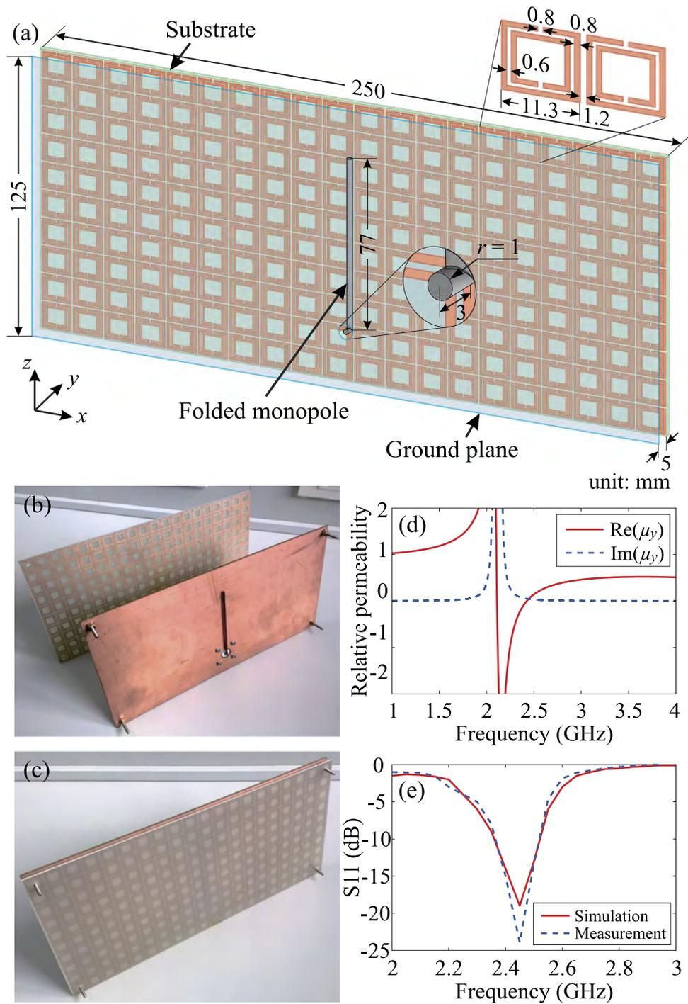
FIG. 3. (a) The configuration of the proposed antenna consisting of a DSRR-HMS and a folded monopole above a ground plane. (b) The fabricated DSRR-HMS and the folded monopole. (c) The complete antenna after two layers are assembled together. (d) The retrieved effective permeability of the DSRR-HMS. (e) Comparison of simulated and measured return loss of the antenna.
