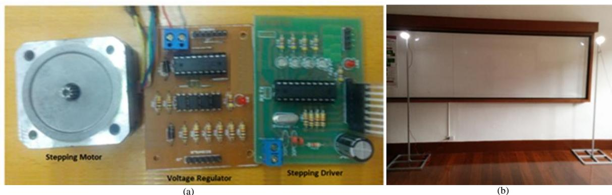
Fig. 3. (a). Motor control unit (b). Experimental setup.
